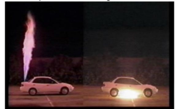
Photo 2 - Time 0 min, 3 seconds - Ignition of both fuels occur. Hydrogen flow rate 2100 SCFM. Gasoline flow rate 680 cc/min.
